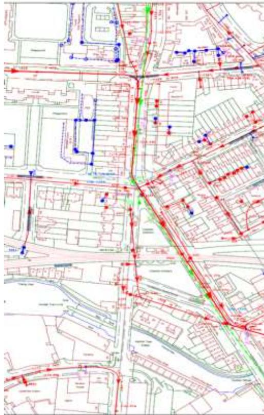
The main sewer line at Kentish Town Road is joined by an oblique 'spur', along the former line of the Fleet, from behind at Farrier Street and runs down Camden Street, turning further east to pass beneath the Regent's Canal. This course is confirmed by a map from development of the site at 25 Camden Road (Shirley House, currently British Transport Police offices), which is between the triangle of Regent's Canal, Camden Street and Camden Road
